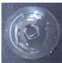
Figure 1 - Size 3 EMBOCAPS® LPR VG Pro post DPI puncture
